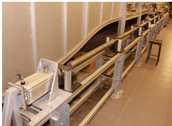
Figure 1: Split Hopkinson pressure bar system used for testing specimens at high strain rates, from about 30 to 300 \text{ s}^{-1}
